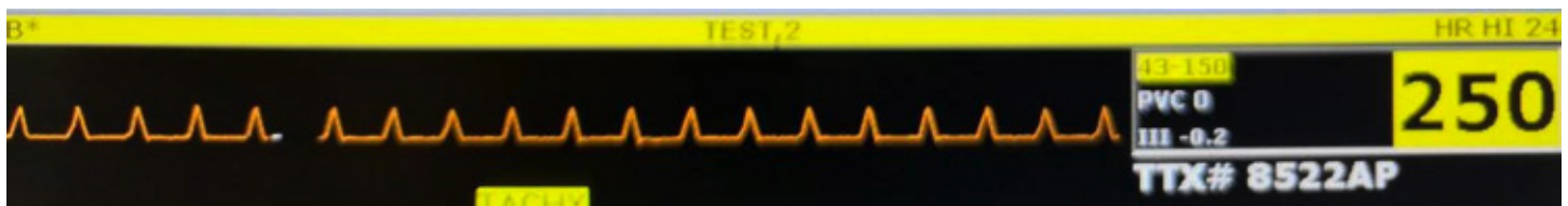
Figure 4: Representative tracing with an AirLife leadwire set with an Input Rate of 250 BPM.
