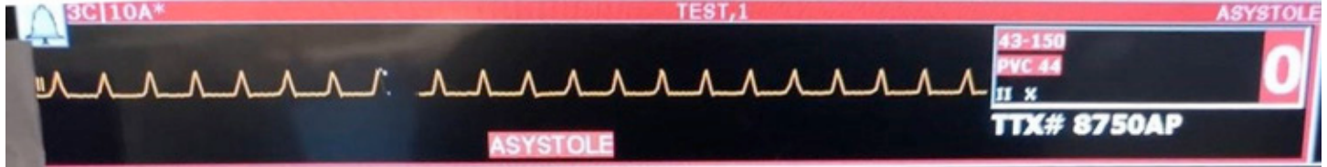
Figure 3: Representative tracing with a Cardinal Health leadwire with an Input Rate of 250 BPM. Note the asystole false alarm with a measured rate of 0 BPM.
