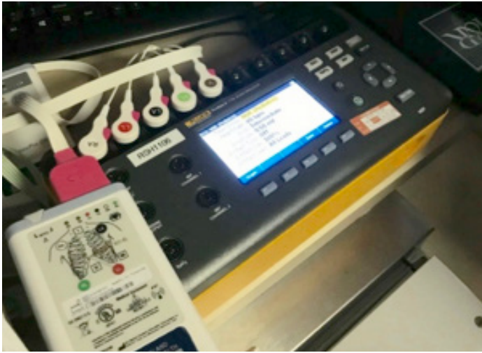
Figure 1: Photograph of example experimental setup. A five-lead snap/grabber combo leadwire set (Cardinal Health) connected to a Vital Signs Simulator (Fluke ProSim 8).
